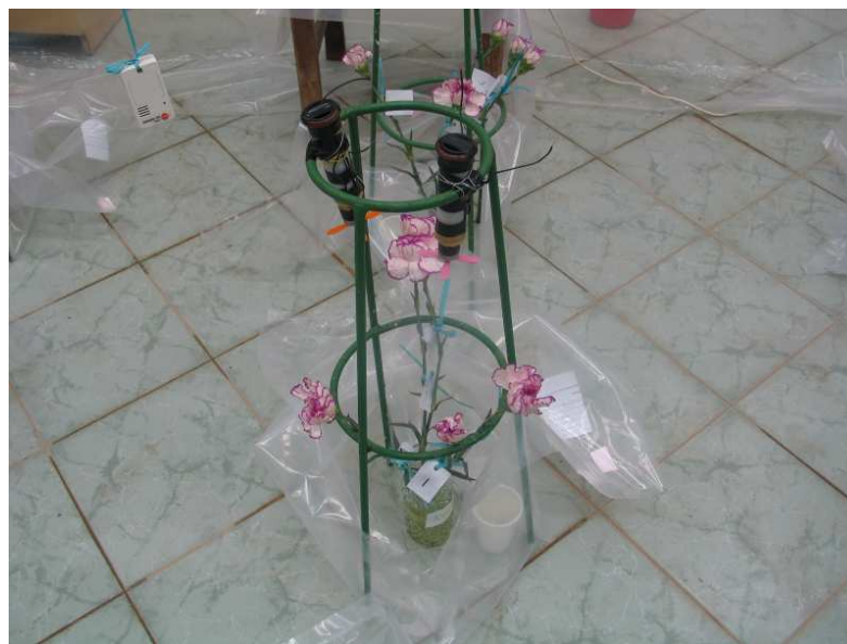
Fig. 1. The support, vase containing cut flowers and air mixing fan set.
