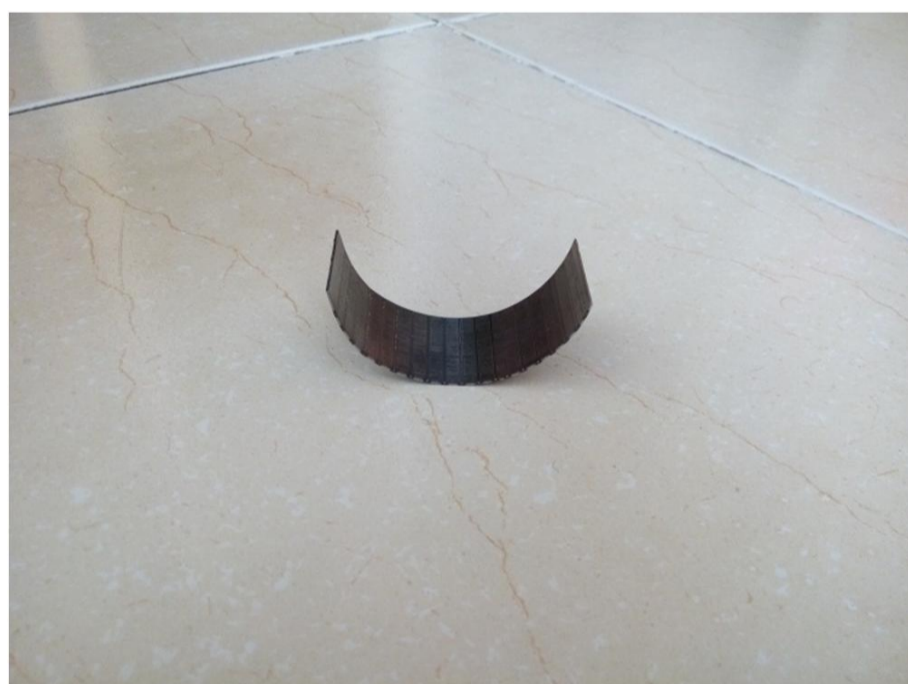
Fig. 3 A sample of cylindrical parts produced by laser and using the proposed method
